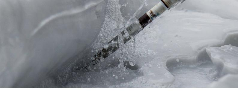
he ROBOTOR project's design philosophy is unique as it applies a gentle approach rather than aggressive action when working with materials. Diamond tips of gradually finer dimensions are used to mill materials, making it possible to use composite materials made from recycled processing waste. This sustainable solution marks the beginning of a new era in stone milling.
